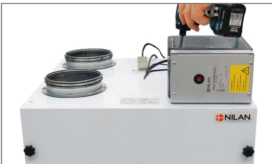
3. The preheating surface is installed at the outdoor air duct connection on the top (standard) or on the side of the unit (in which case the cover plate must be moved to cover the hole in the top). Be sure to place the heating surface so that the cover for the automatic opening can be easily opened.
